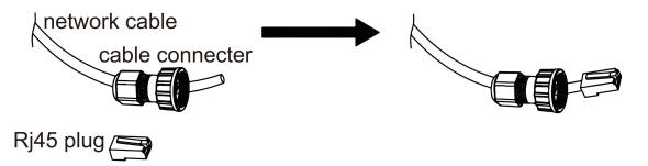
Step 4: Insert the cable connector into COM port at the bottom of energy station and screw it tightly. Then insert other side of the network cable into PC or another device.
