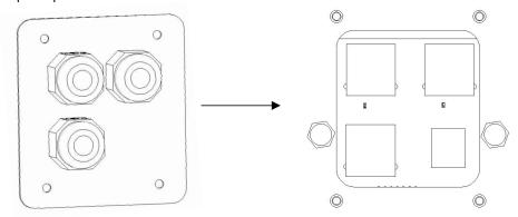
Step 2: Prepare a standard network cable and cable connector, then insert the network cable through the cable connector.
