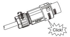
• Push the threaded sleeve to connection terminal until both are locked tightly on the energy station.
