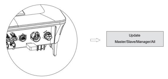
d. Short press on the button to select the type of firmware you want to upgrade, then long press on the button, the inverter will start the upgrade process automatically.
