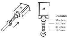
3.Crimp the cold-pressed terminals. To ensure insulation between the terminals, please sleeve the crimped section of the cold-pressed terminals with heat shrink tubing and heat it for tight fitting to prevent the tubing from loosening.
