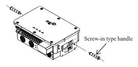
2.Install the inverter on the hanging plate, and ensure that slots of the inverter are properly matched with the hanging plate.
