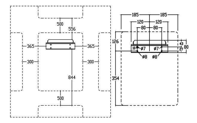
Before drilling holes, please ensure the distance between the machine and nearby objects.
