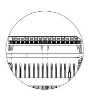
Please keep the top of filter flush with the back of inverter. Please adjust to the position where the lateral fins can be seen from the holes on both sides of the filter according to the figure in which the arrow towards to the wall.
