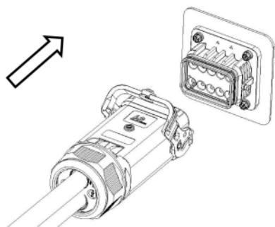
After the male and female insert the card point into the tracks lot, press the lock.
