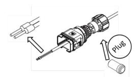
Insert the wires into the corresponding terminals.
