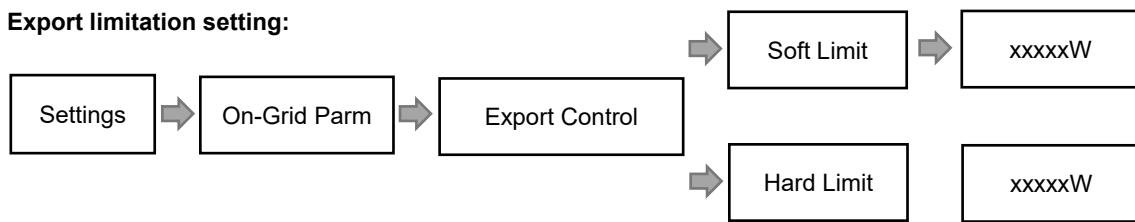
After enabling Export Control, the inverter will respond to the export power control in real time according to the CT or meter to control the active power export level. By default, the Export Control function is disabled.
