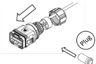
Lock wire nut screwed onto the body, torque  $2.5+/-0.1\text{N}\cdot\text{m}$ , then complete installation.
