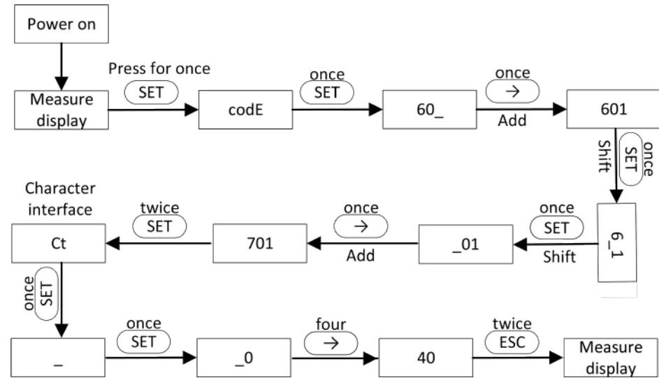
The address of the second meter is 2. Please ensure that the address is 2, otherwise the communication of the first meter will be affected, and the output and monitoring data of the inverter will be affected.
