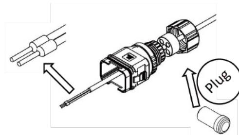
Insert the wires into the corresponding terminals.
