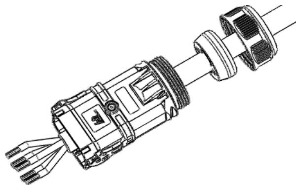
First, insert the EPS end cable into the EPS end of the rubber core. After the cable is in place through the perspective hole, tighten the screw using an S2.5 hexagon wrench with a torque of  $2.5\pm0.1\text{N}\cdot\text{m}$ .
