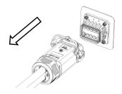
PV and BAT disassembly diagram
