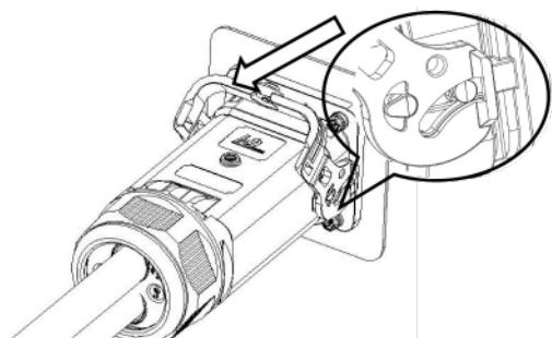
Tighten the screws with the S2.5 hexagon wrench with a torque of  $2.5\pm0.1\text{Nm}$ . Installation completed.
