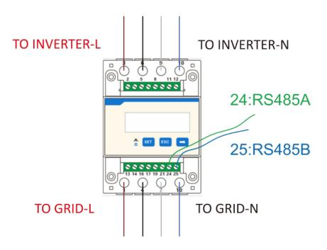
Insert L1/L2/L3/N wires and RS485A/B cable into the meter. Please refer to the meter wiring diagram on side of meter itself.
