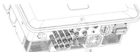
1. Press the connector buckle at the BAT side;
