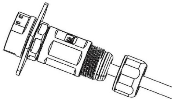
Tighten the connector's nut by the open-ended wrench with a torque  $1.2\pm0.2\text{N}\cdot\text{m}$ .
