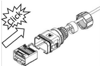
Install the plug into the main body and plug the holes without wires with a plug.
