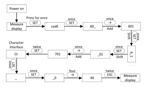
The address of the second meter is 2. Please ensure that the address is 2, otherwise the communication of the first meter will be affected, and the output and monitoring data of the inverter will be affected.
