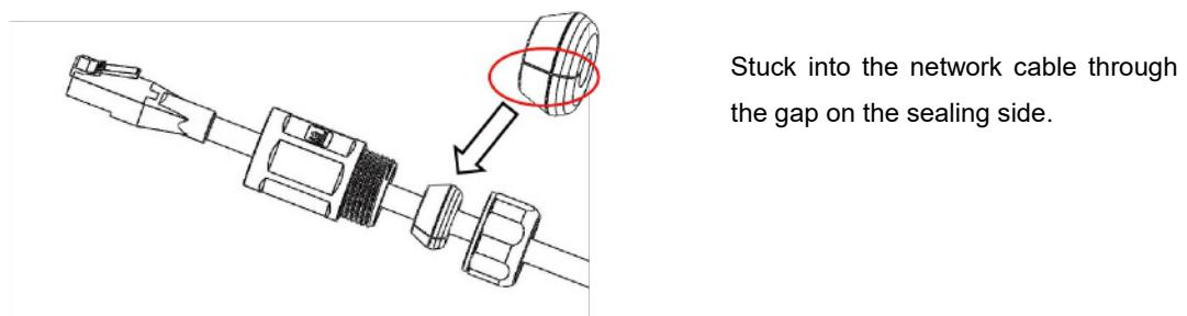
Insert the network cable plug into the matched RJ45 panel mount connector.
