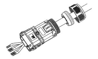
First, insert the EPS end cable into the EPS end of the rubber core. After the cable is in place through the perspective hole, tighten the screw using an S2.5 hexagon wrench with a torque of 2.5±0.1N·m.
