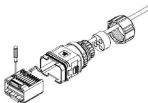
Arrange the core line, the rubber core area must not appear to ride the line. The rubber core is loaded into the main body and accompanied by a "click" sound.
