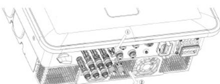
1. Press the connector buckle at the BAT side;
