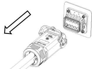
PV and BAT disassembly diagram
