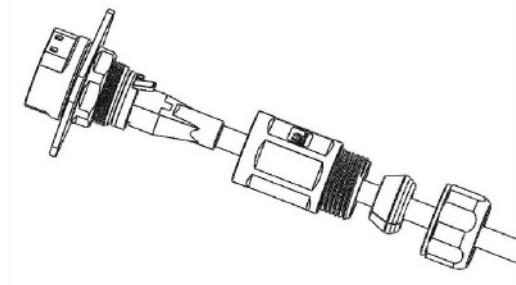
Tighten the connector mainbody by the open-ended wrench into the RJ45 panel mount connector with a torque  $1.2\pm0.2\text{N}\cdot\text{m}$ .
