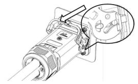
Tighten the screws with the S2.5 hexagon wrench with a torque of 2.5±0.1Nm. Installation completed.
