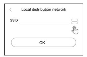
Step 3: Connect your mobile device with Smart WiFi. The SSID of the Smart WiFi is 'W-xxxxx' and the password is 'mtmt2020'.
