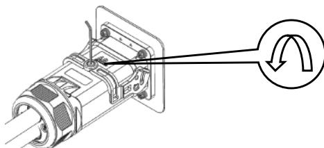
2. Open latch to unlock position (about 45°)
