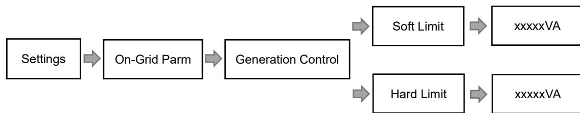
After enabling the Generation Control, the inverter will response to the generation power control in real time according to the CT or meter to control the apparent power level. By default, the Generation Control function is disabled.
