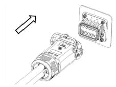
After the male and female insert the card point into the tracks lot, press the lock.
