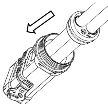
Tighten the nut with an open-ended wrench. (torque  $10.0\pm0.1\text{N}\cdot\text{m}$ , Complete the installation)
