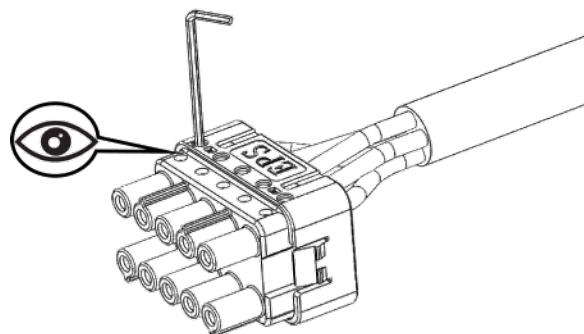
Insert the GRID end-core wire into the GRID end of the rubber core, observe the perspective hole cable in place, use S2.5 hex wrench to tighten the screws, torque  $2.5\pm0.1\text{N}\cdot\text{m}$ ;
