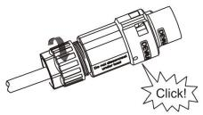
• Push the threaded sleeve to connection terminal until both are locked tightly on the inverter.
