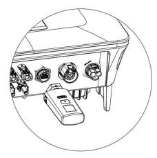
c. Wait until the LCD is off, then insert the U-disk to "WiFi/GPRS/4G/USB" port and turn on the DC switch or re-connect the PV connector, the LCD will show picture as below.
