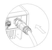
• Remove the AC connector, press the bayonet out of the slot with a small screwdriver or the unlock tool and pull it out, or unscrew the threaded sleeve, then pull it out.
