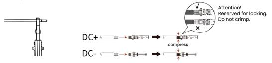
• Insert pin contact through the cable nut to assemble into back of the male or female plug. When you feel or hear a "click" the pin contact assembly is seated correctly.
