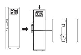
Insert 2 pcs of M5×30 screws (F2) into the holes on the left and right sides of the mounting bracket then tighten the screws.
