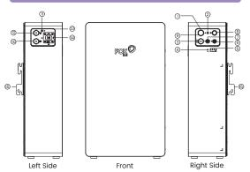
Handle (9) Valves 2 **Ground Terminal** (10) LINK OUT 3 Ground Terminal PCS COM (11) 4 BMS Status LED (12) LINK IN (5) BMS SOC LED (13) Handle (6) DC+ (14) DC Switch (7) (15) **Battery Bracket** DC-(8) Power Switch
