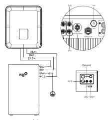
Note: Power Cable (L2) must be pulled straight from the battery DC+/- for more than 80mm before bending.
