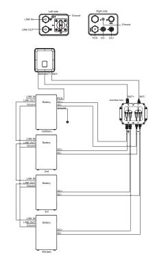
Note: Keep a distance of 300-600mm from the battery to the junction box. Power Cable (L2) must be pulled straight from the battery DC+/- for more than 80mm before bending.
