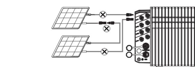
4. If you want to disconnect the PV connector: After ensuring the system is turned off, use the included wrench to safely remove the PV connector.
