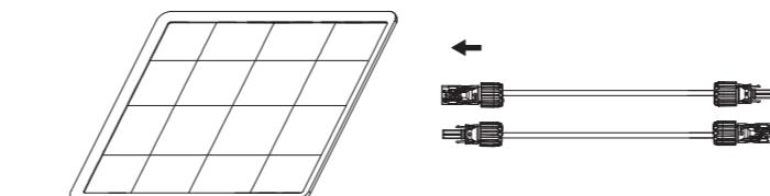
3. Connect each PV module directly to the same set of PV input ports.
