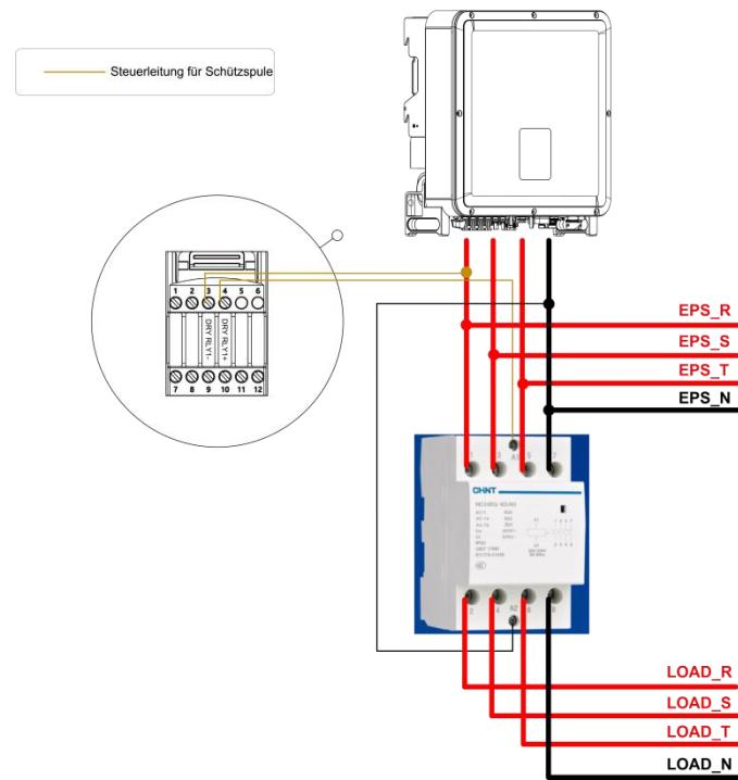
DryConfigure setting: DryConfigure Set the DryOut1 to Smart EPS.
