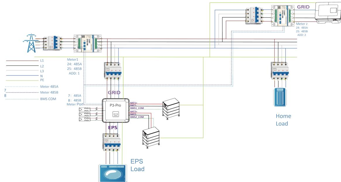
Important: Supports the function of the second electricity meter, which is used to measure the power generation of other power generation equipment and to summarize the monitoring data on the website.
