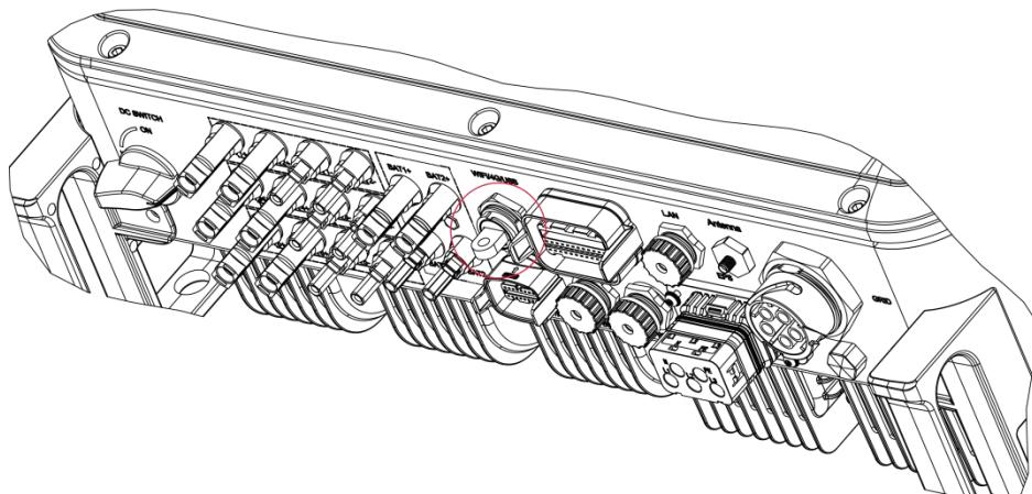
4. Only turn on DC breaker (**make sure PV voltage is above 120V**) wait for 10 seconds, the inverter screen will show as below:
