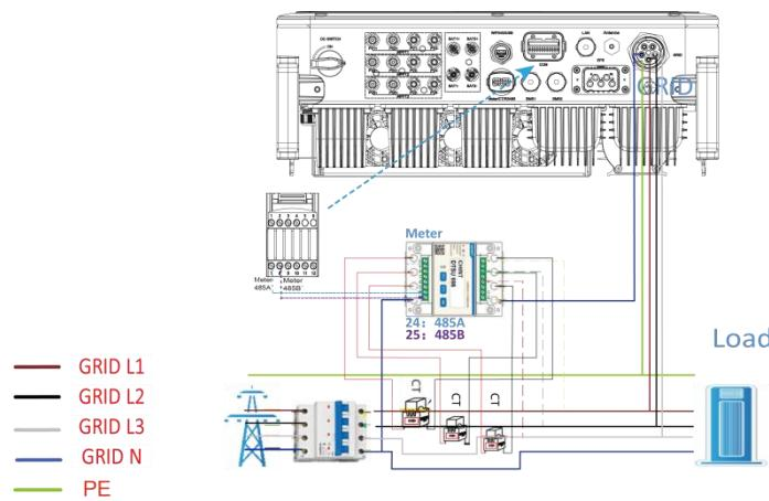
Insert L1/L2/L3/N wires, CT and RS485A/B cable into the meter. Please refer to the meter wiring diagram on side of meter itself.
