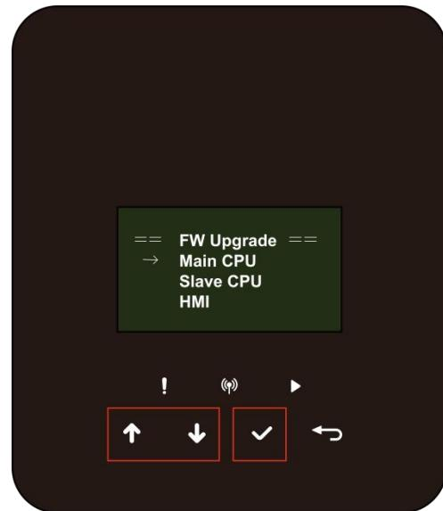
6. Remove the USB disk after upgrade completed. Follow the procedure blew and click the option to view the version:
