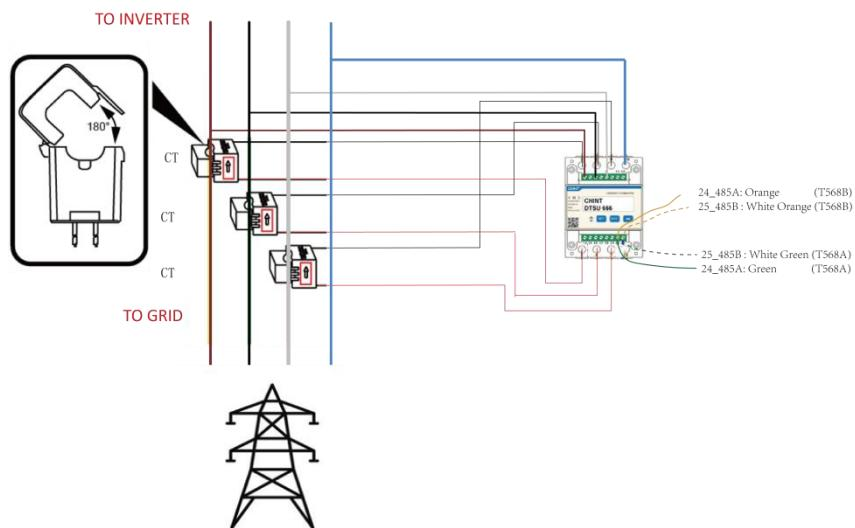
Notes: The 2,5,8 of the CT meter are connected to the three live wires L1, L2, and L3 respectively.
