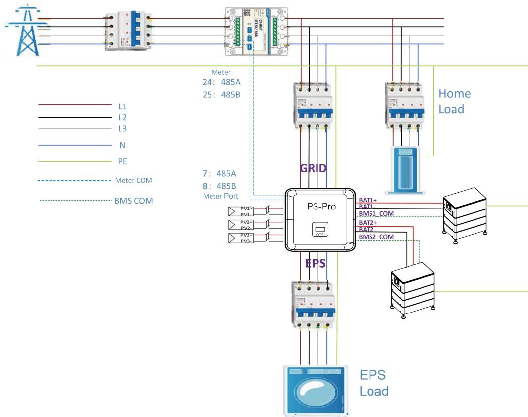
Important: P3-Pro needs to be connected to the 3-phase 5-wire power grid system, and ensure that the GRID is connected to the N line, otherwise the machine will report the SW BUS VOLT fault.
