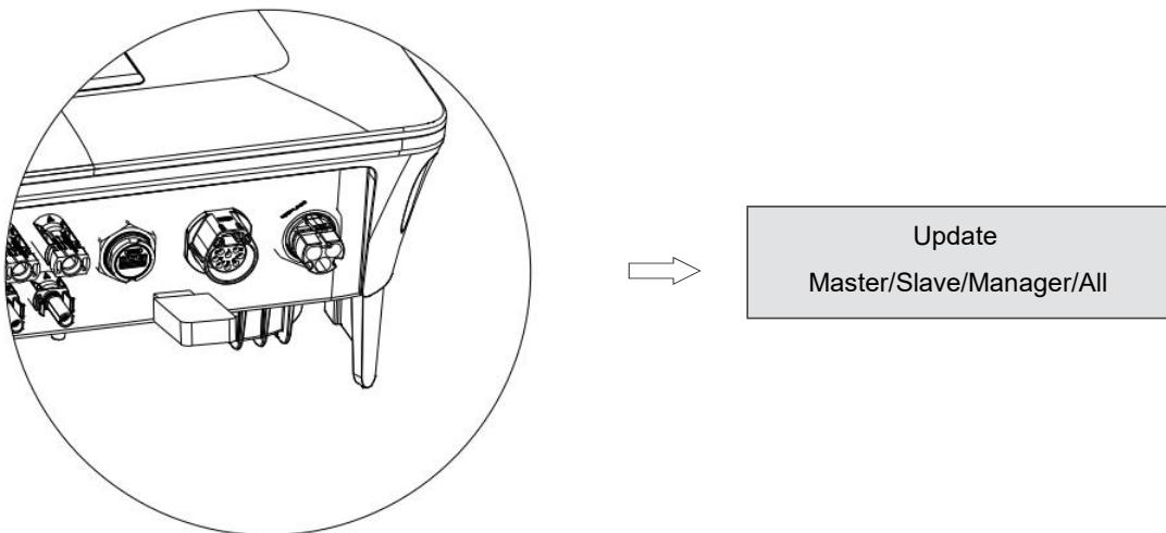
d. Short press on the button to select the type of firmware you want to upgrade, then long press on the button, the inverter will start the upgrade process automatically.
