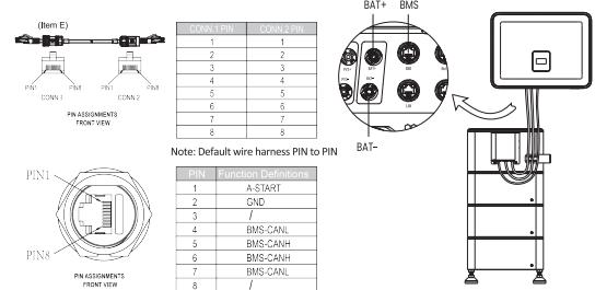
**Note:** If using a new RJ45 cable, the waterproof union nut can be removed from the communication cable (Item E) and placed into the new cable to ensure proper sealing.
