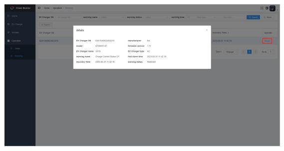
If the charging pile fails, alarm data will be generated in the alarm message module. Click on the Details button to view the alarm details of the charging pile.
