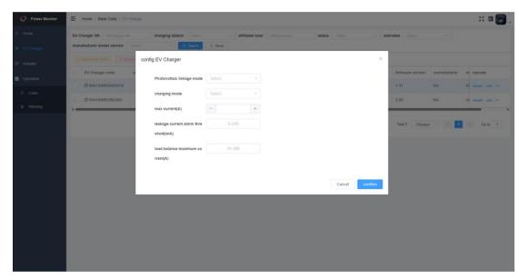
When the charging pile is in standby and connected state, click the Configure button. You can set the PV linkage mode, charging mode, maximum current, leakage current alarm threshold, load balancing maximum current.
