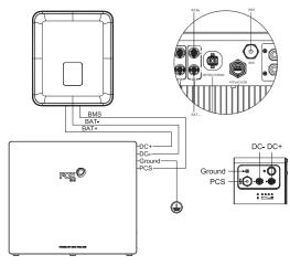
Note: Power cable (K2) must be pulled straight from the battery DC+/- for more than 80mm before bending.
