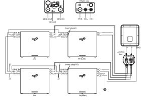
Note: Keep a distance of 300-600mm from the battery to the junction box. Power cable(K2) must be pulled straight from the battery DC+/- for more than 80mm before bending.
