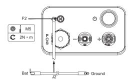
b. Connect the PCS communication cable (I2) to the BMS port on the inverter.
