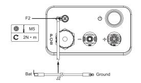
**b.** Connect the PCS communication cable (I2) of the **Main** battery to the BMS communication port of the inverter.
